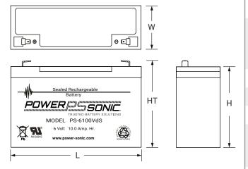
**L**: 5.94 (151) **W**: 2.00 (51) HT: 3.93 (100) **H:** 3.70 (94) Tolerances are +/- 0.04 in. (+/- 1mm) and +/- 0.08 in. (+/- 2mm) for height dimensions. All data subject to change without notice.
